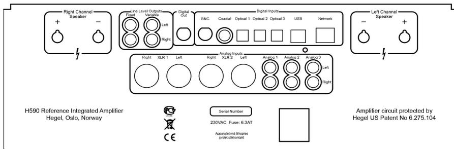
Always power the amplifier off before connecting input/output audio cables and the power cable.
