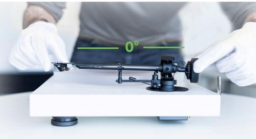
**14** Turn the front scale of the counterweight to Zero without moving the weight itself.
