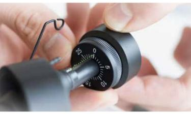
Turn the whole counterweight counterclockwise until the scale reads 18 - 20.
