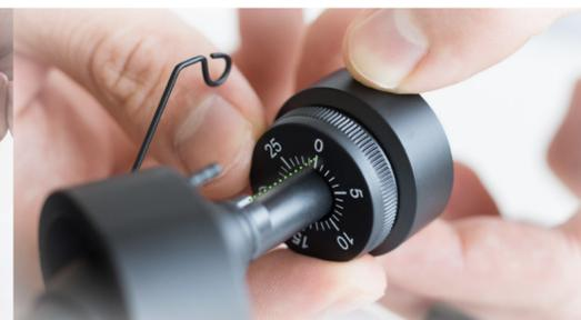
**19** Turn the whole counterweight counter-clockwise until the scale reads 18.
