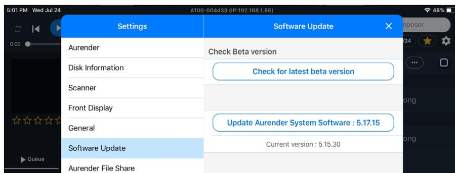
Note: Conductor will temporarily lose connection to the Aurender as the unit reboots during the upgrade process. Please quit the Conductor app and reopen once the upgrade has completed.
