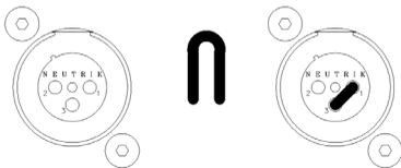
Figure 7: XLR connector without and with jumper accessory
