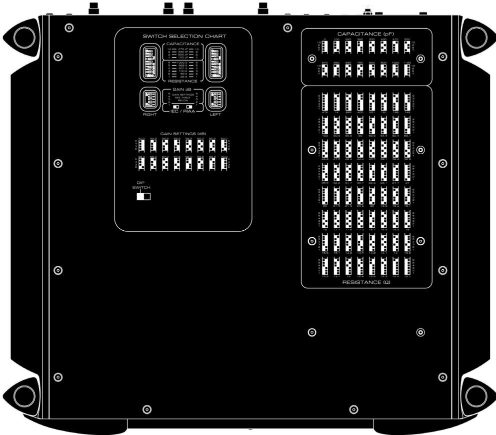
Settings for cartridge resistance loading, cartridge capacitance loading, gain and equalization curve are all done using white colored DIP switches located on the 610LP's bottom panel as shown above in figure 1. There are two (2) banks of DIP switches – The upper bank provides for the capacitance and resistance loading adjustments; the lower bank for gain level and equalization curve settings.
