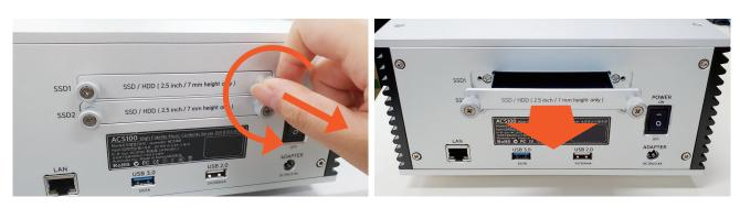
1. Unscrew and eject the disc enclosure tray[s] before turning the unit on.
