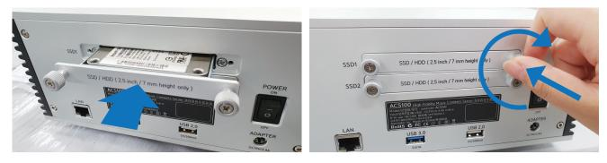
3.Gently push the tray[s] containing SSD[s]/HDD[s] into the slot. After tray is in position, turn screws clockwise to secure tray.
