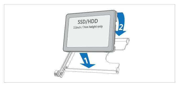
2.Install SSD[s]/HDD[s] into the tray[s] as pictured.
