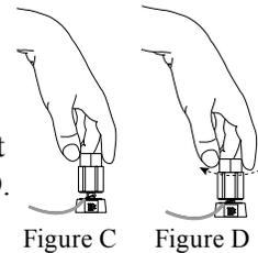
3. Rotate the top of the Output Terminal Post clockwise until it is finger tight. Refer to figure D.
