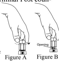
2. Insert the Loudspeaker hookup cable into the Output Terminal Post opening or the cable spade lug around the center post of the Output Terminal. Refer to figure C.
