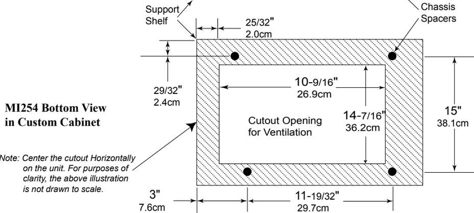
Note: Center the cutout horizontally on the unit. For purposes of clarity, the above illustration is not drawn to scale.
