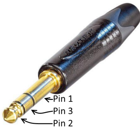
Figure 7: Neutrik balanced jack connector
