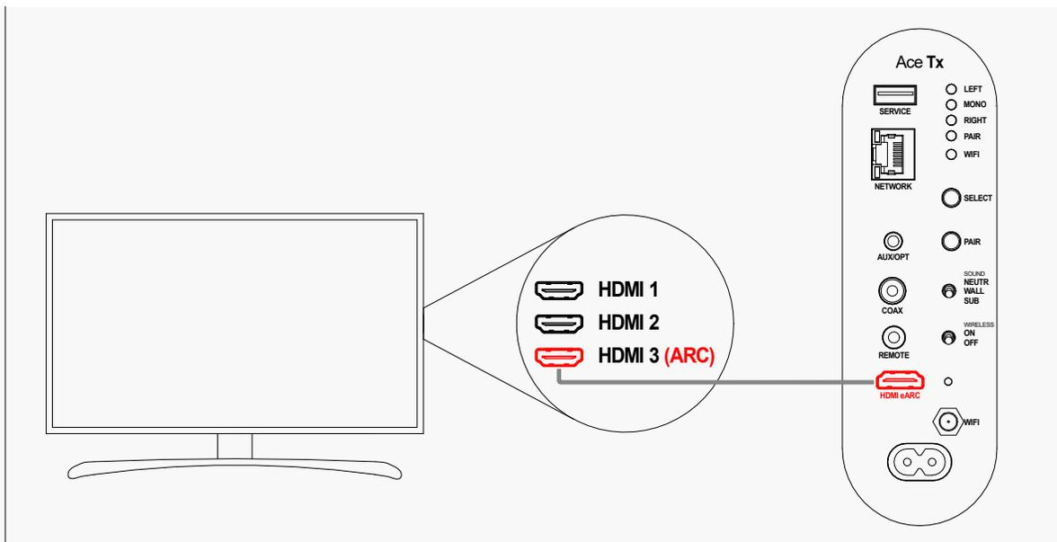
Double-check the settings on your TV to make sure the sound is played back through the HDMI ARC output.
