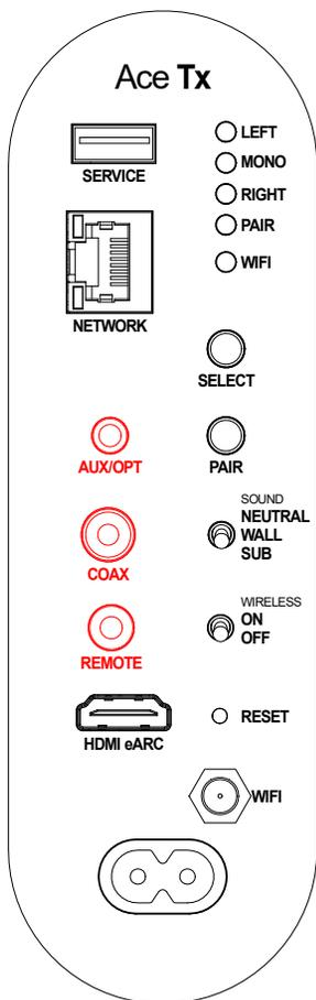
**Note:** For both options use the «AUX/OPT» jack on the rear panel. A corresponding adapter for the optical connection is included in the scope of delivery.
