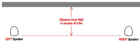
**WALL:** Flip the switch to «WALL» for speakers positioned less than 50 cm from the wall. In this setting bass tones below 100 Hz are reduced.
