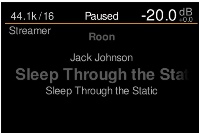
When turning the MU2 main control knob, the volume changes and the track progress bar at the bottom is temporarily replaced by a bar that indicates the current volume setting. You will hear the relays of the analog volume control clicking inside the MU2 box when you change the volume.
