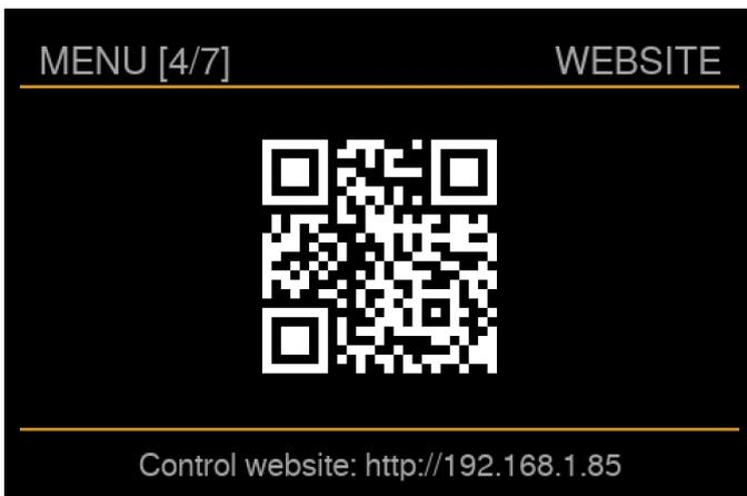
This menu shows the information you need to connect to the Grimm User Interface (GRUI). The GRUI is the web control interface of the MU2. You can scan the QR code with your tablet or mobile device. As an alternative you can manually enter the link shown at the bottom of the screen in your browser. More information about the GRUI can be found in chapter GRUI MU2 Web Control. This menu page will automatically be shown at maximum screen brightness for optimal scannability.
