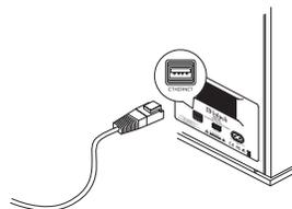
Figure 3– Ethernet connection
