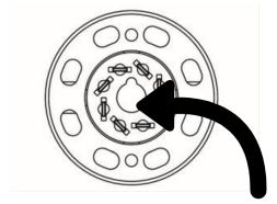
Some tubes, including the 5AR4 rectifier tubes in your EvoLotion Series Preamplifier, have a "center locating key" which must line up with the socket! If you misalign them and use brute force to push the tube in place, you will damage important and expensive parts of your preamplifier! This damage will void your warranty so use caution when installing power tubes!
