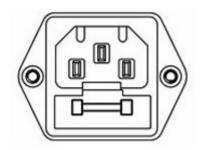
Mains Fuse: The mains fuse is located on the rear of the amplifier, just below the power cord socket (see picture on the left). The fuse rating is 1 x Littelfuse 213 Series 3.15A Slow Blow 5 x 20mm fuse for 100-125VAC and Littelfuse 213 Series 1.6A Slow Blow 5 x 20mm fuse for 200-250VAC. Always replace with the same type and value fuse! The fuse holder can be opened using a small slotted flat blade screwdriver.
