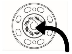
Many tubes, including all power tubes that can be used in your EvoLution Integrated Amplifier, have a "center locating key" which must line up with the socket! If you misalign them and use brute force to push the tube in place, you will damage important and expensive parts of your amplifier! This damage will void your warranty so use caution when installing power tubes!
