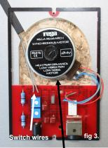
Motor orientation & wiring correctly dressed. Not contacting the motor body
