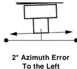
More importantly, this azimuth error will not allow proper tracing of the grooves resulting in mistracking. An edgy, hyper-detailed high-frequency sound will result if the azimuth is set wrong.
