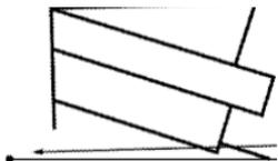
**$1.2^\circ$  Negative Cartridge Rake Angle**
