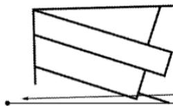
**$1.5^\circ$  Negative Cartridge Rake Angle**
