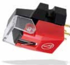
Standard model with a MicroLine® stylus. Distortion is low even on the inner circumference of a record because the curvature radius of the stylus tip does not alter even if the stylus becomes worn.
