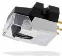
Model dedicated to 78 rpm records, whose round stylus has a large curvature radius at the tip. The curvature radius is 3 mil, and suitable for playing 78 rpm records from a wide variety of eras.
