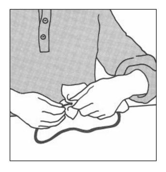
BELT. The belt should last for at least five years of regular use. The belt can be cleaned at the same time as the pulley is cleaned. The best method of cleaning a belt is by pulling it through a damp cloth.
