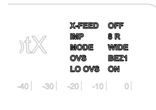
**X-FEED** Indicates whether the cross-feed function is *ON* or *OFF*.
