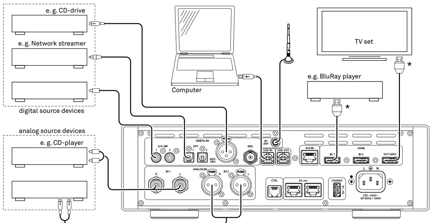
\* Only possible with optional available factory-installed HDMI module
