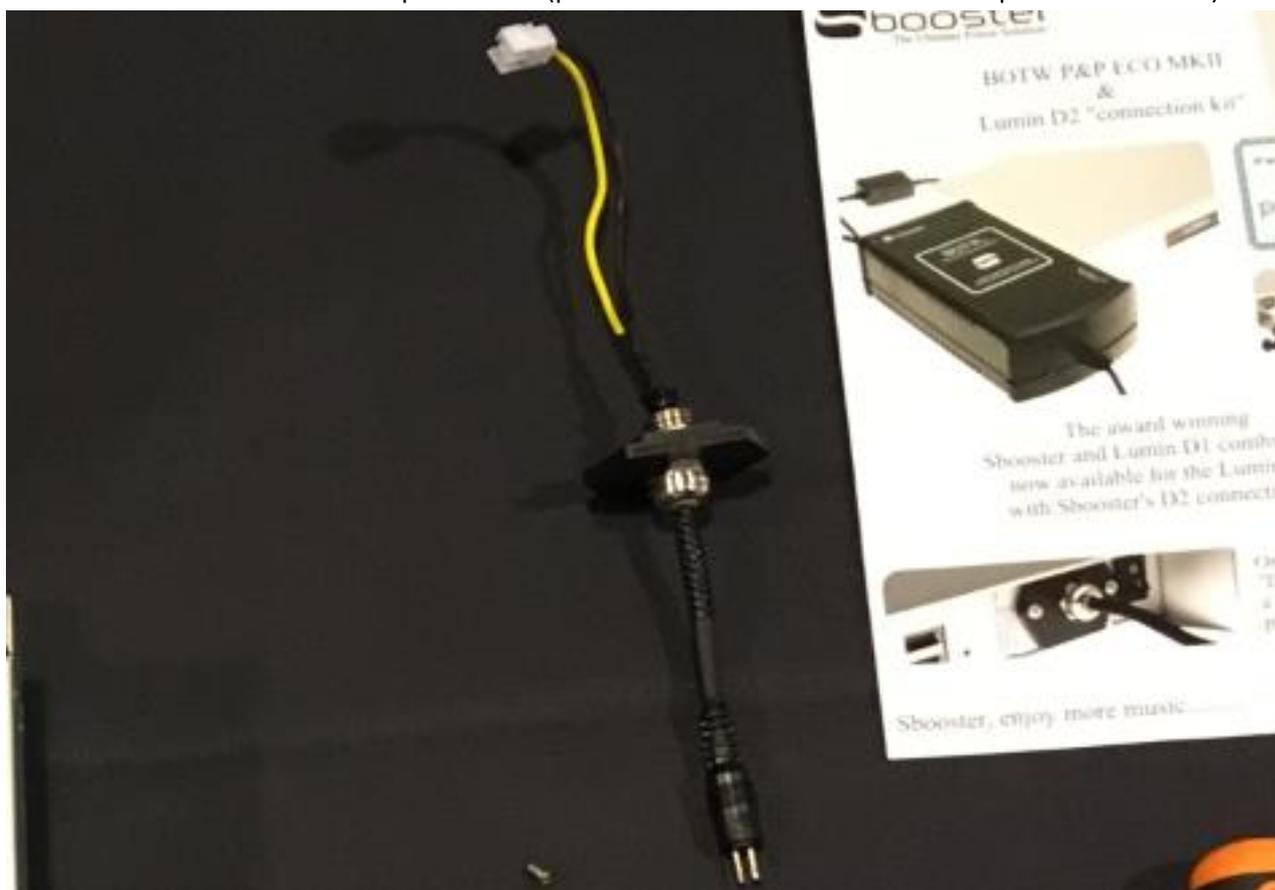
Place the bracket, the Sbooster logo facing up, and fix the unit with the two supplied silver screws.
